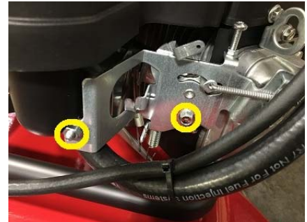
Remove Circled Nut and Bolt
